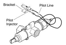
Figure 17 - Installing Propane/LP Pilot Orifice
